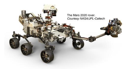
NASA's next Mars rover will collect soil samples, seal them and deposit them on the Martian surface for future collection and transport back to Earth. Swiss manufacturer maxon motor supplies several drives specifically developed for the task.
