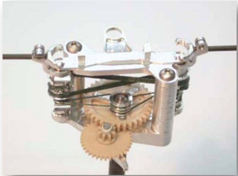
Figure 2 b: The final string-based large amplitude flapping mechanism for the Nano Hummingbird aircraft was made with an aluminum frame and PEEK gears.
