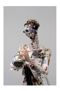
"ECCE Robot" with artificial muscles, driven by maxon motors.
